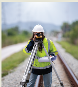
FIGURE 2.2.8 Surveying the land with a theodolite.
