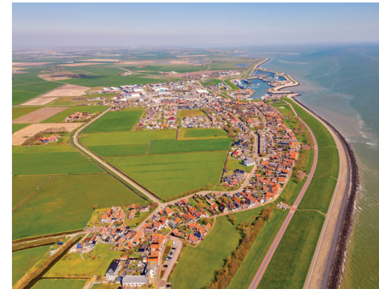
6.1.4 Dyke protected, reclaimed polder in the Netherlands
