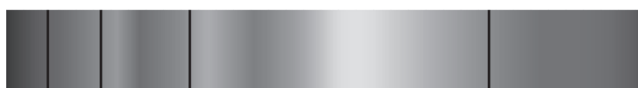
FIGURE 1.1.10 Absorption spectrum for hydrogen. The energy levels of the black lines on what would be a coloured background correspond to the energy levels of the coloured lines on the background of the emission spectrum.
