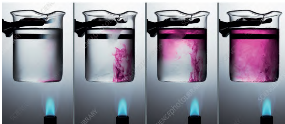
FIGURE 2.3.6 Demonstration of convection using a Bunsen burner, water and food colouring
