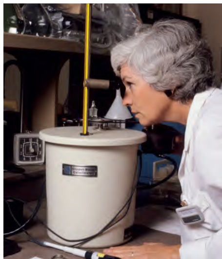
FIGURE 2.6.1 A scientist uses a bomb calorimeter to measure a temperature change to determine the thermal energy transfer.
