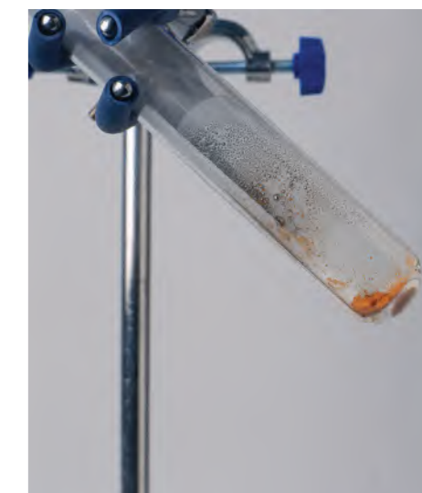
FIGURE 2.1.10 The red powder in this test-tube is mercury(II) oxide (HgO). If you look closely at the test-tube, you will see beads of liquid mercury forming from the decomposition of the compound.
