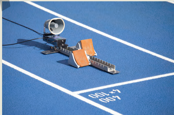
FIGURE 3.1.4 Starting blocks are fitted with pressure sensors to detect false starts.
