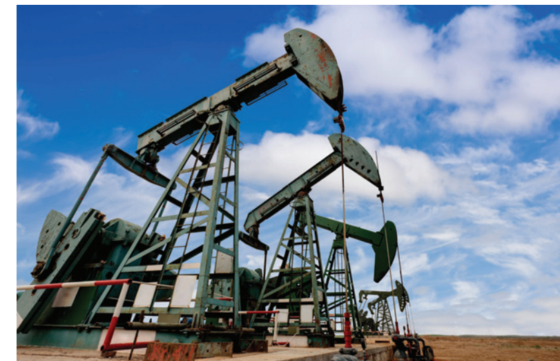
5.1.3 A pumpjack on an oilfield that mechanically lifts the oil out of the well if there is not enough pressure for it to flow up to the surface from the reservoir below.
