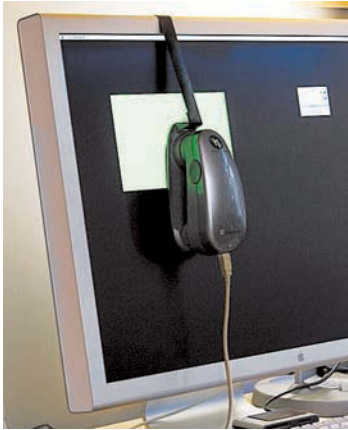
Figure 4.1 I normally use the X-Rite i1Photo to calibrate the displays I use at work.
