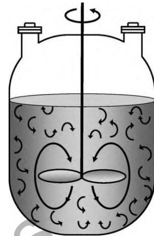
Figure 1-5(b) Batch reactor mixing patterns. Further descriptions and photos of the batch reactors can be found in both the Visual Encyclopedia of Equipment and in the Professional Reference Shelf on the CRE Web site.
