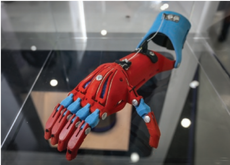
Figure 1.13 3D printing has become a tool for developing more inexpensive, and more stylish, prosthetic devices. (Cem Ozdel/Anadolu Agency/Getty Images)
