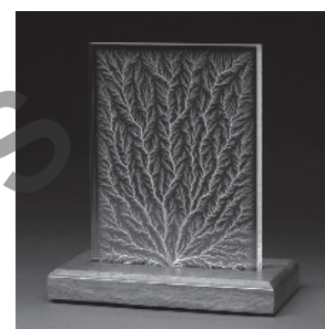
FIGURE 20.26 Dielectric breakdown in a solid piece of Plexiglas produced this striking fractal pattern that marks permanent changes in the material.
