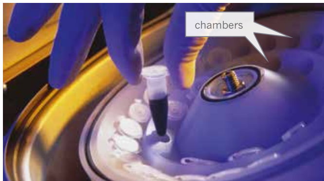
FIGURE 4.2.9 A simple centrifuge is used to separate substances in the laboratory.
