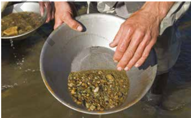
FIGURE 4.2.2 Panning for gold uses gravity separation.
